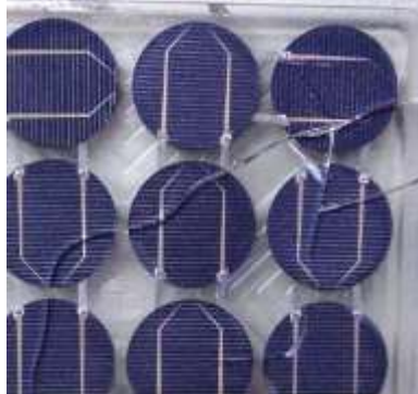
Fig.3: Heat dissipated in a shaded cell caused the module to crack.
